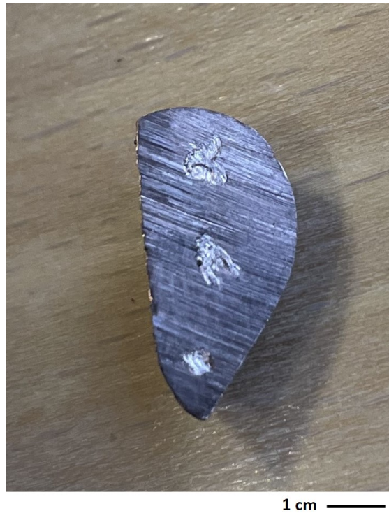
Figure 34: Cross section view of the prepared alloy with Cu 95 at. % and Ag 5 at. %.
